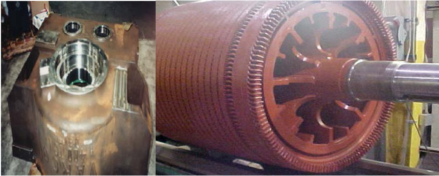
Oversized Bearing housings. Electric Motors
