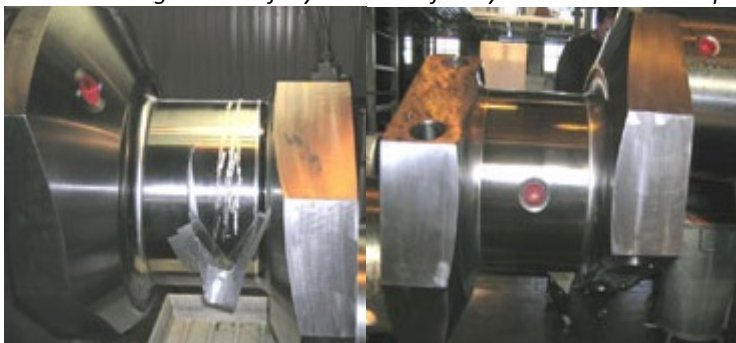
Crankshaft Crankpin damaged and repaired afterwards.
