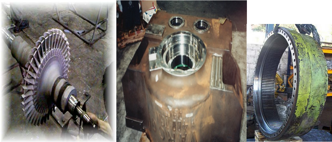
Turbo Wheels and Housings. Oversized Bearing housings restored to OEM specs, among others...
