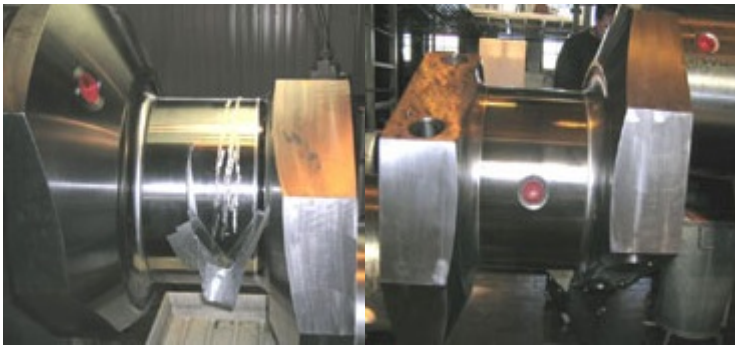
Crankshaft Crankpin damaged and repaired afterwards.
