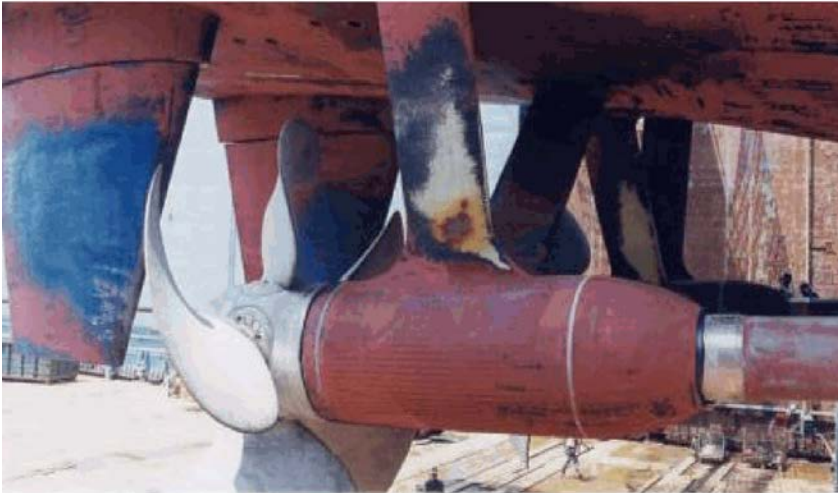
Undersized tail shafts restored.
