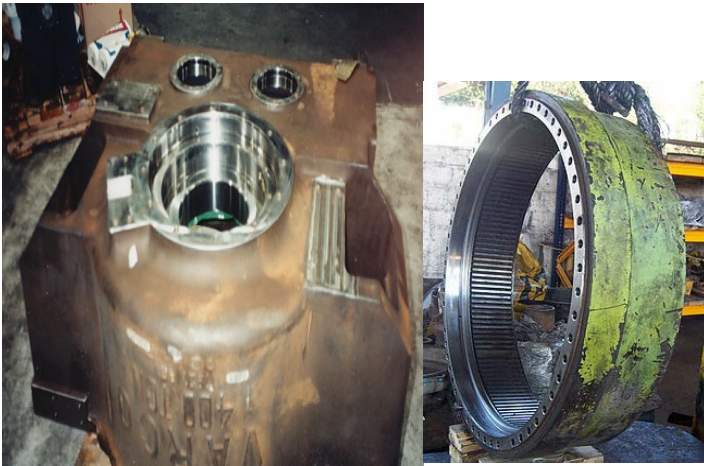
Oversized Bearing housings restored to OEM specs, among others...
