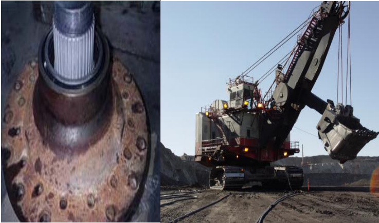
Dragline (Shovel) oversized bush housings and sprocket drives restored.
