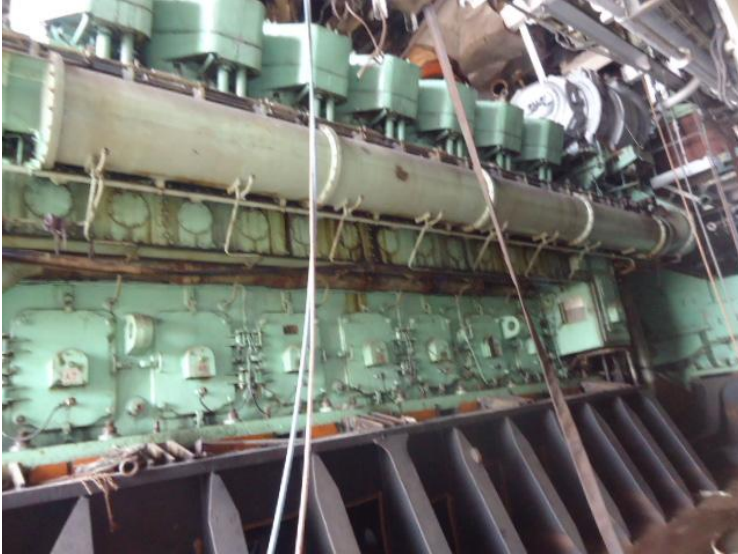
Engine Block (4,300 KW), fully restored.
