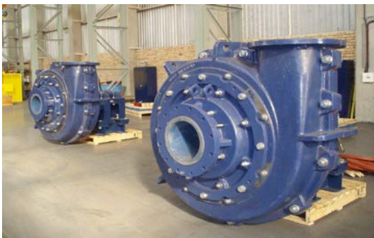
Skurry pumps restorations – impellers, casings, abrasion resistance...
