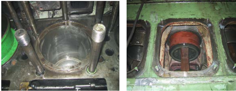
6 MW HFO Engine Block fully restored after cylinder area catastrophic failure.
