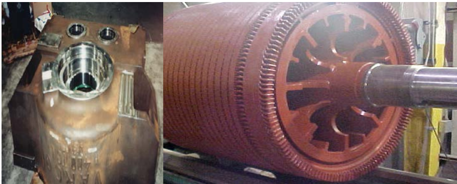
Oversized Bearing housings. Electric Motors
