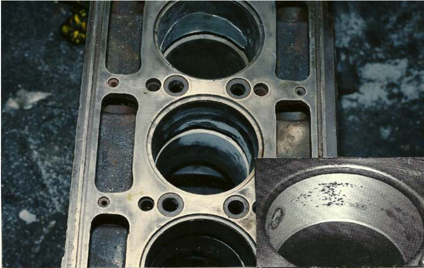
Engine Block (1,200 KW) showing cooling port damages, fully restored.
