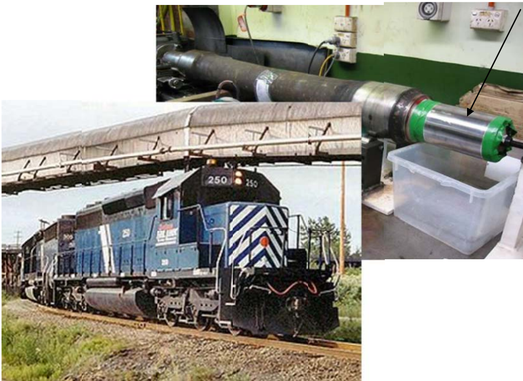
Undersized bearing areas on shafts restored.
