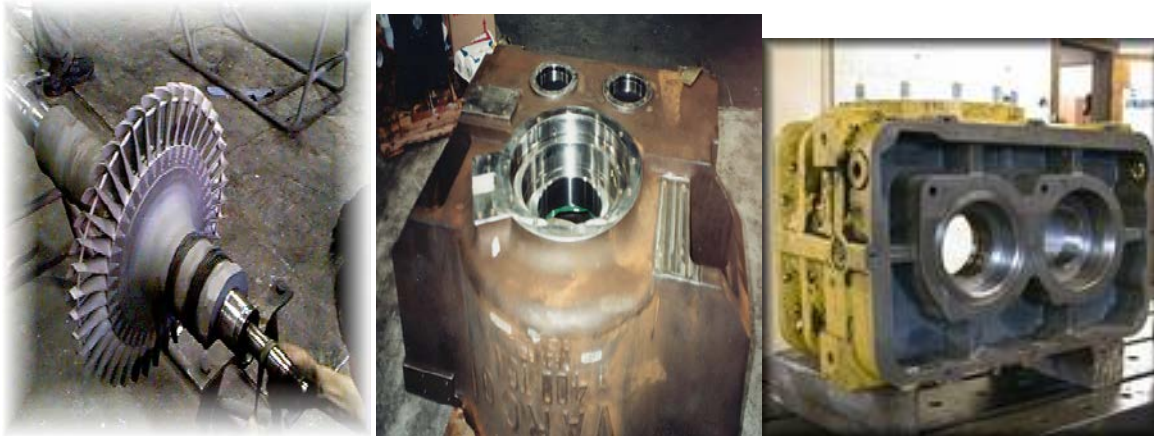
Turbo Wheels and Housings. Oversized Bearing housings restored to OEM specs. Minority owned and operated.
